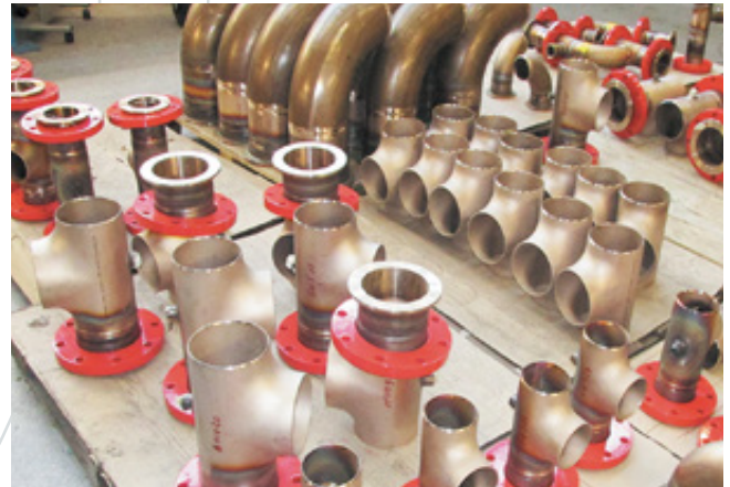
90/10 CuNi piping spools
