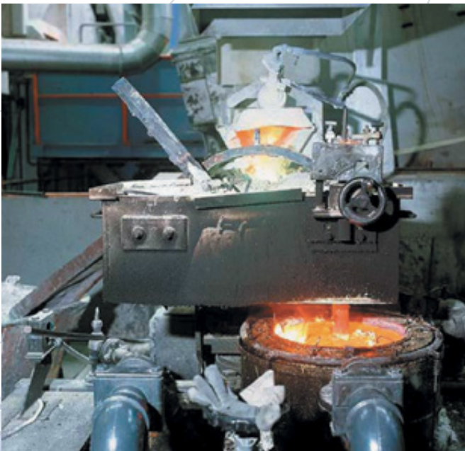
Semi continuous casting of CuNi billet
