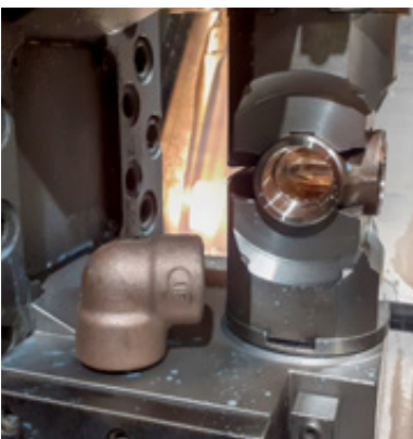
90° socket weld elbow machining
