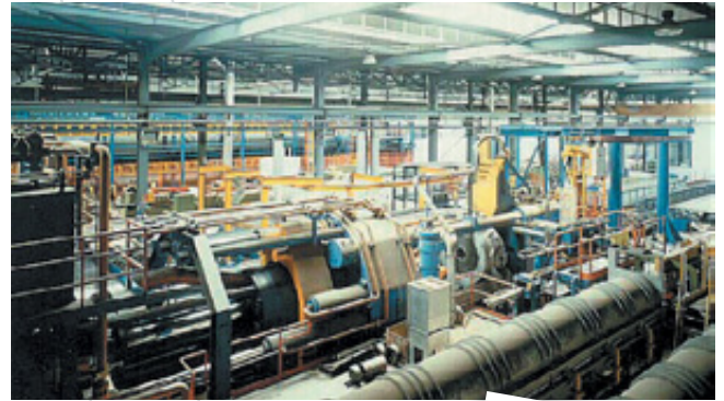
5500 tons Hot Extrusion press
