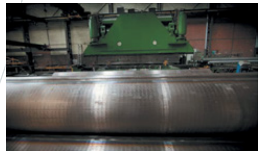
U-BEND PRESS CuNi pipe forming
