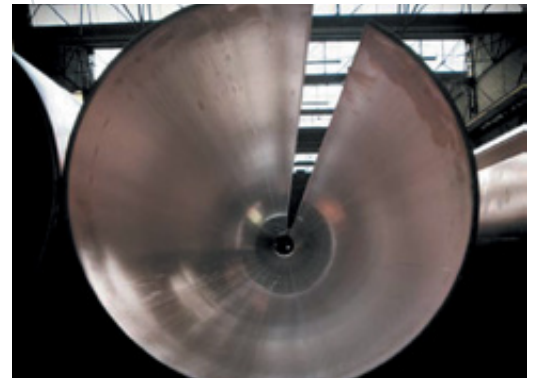
3 ROLLS CuNi pipe forming
