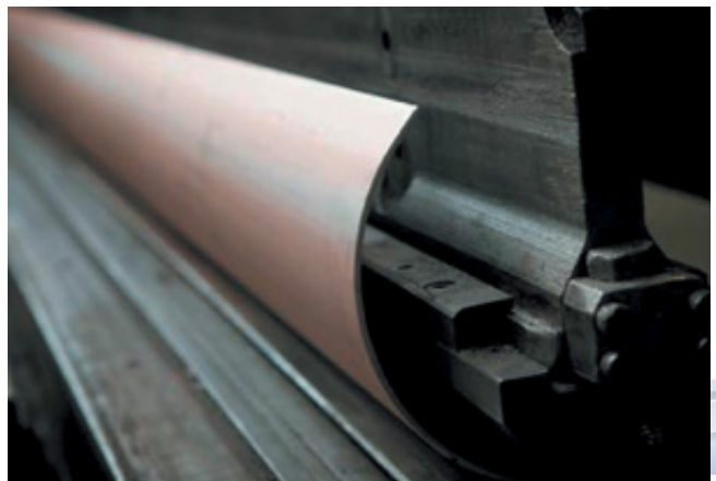
U-BEND PRESS forming CuNi plate into pipe
