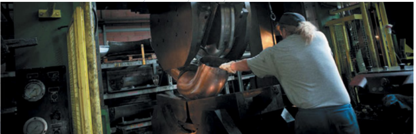
Cold forming CuNi elbows from seamless pipes
