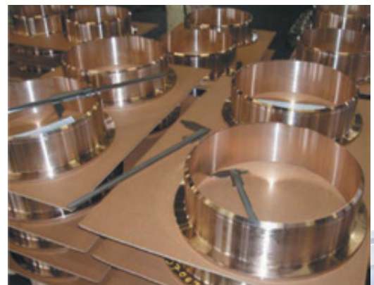
CuNi Inner flanges final inspection
