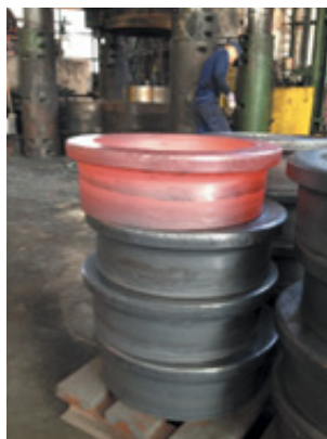
Hot forging of 20" CuNi stub ends
