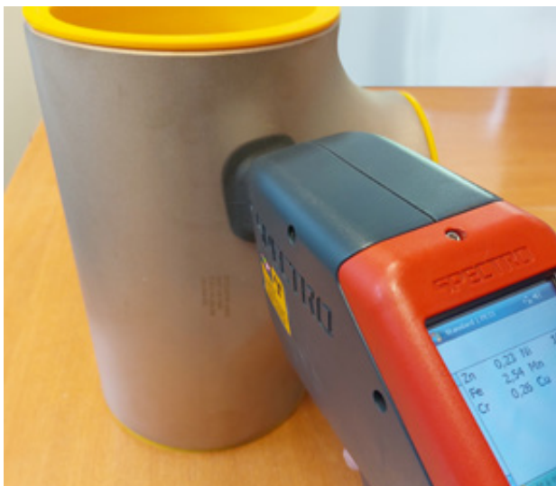
Positive Material Identification Test (PMI)
