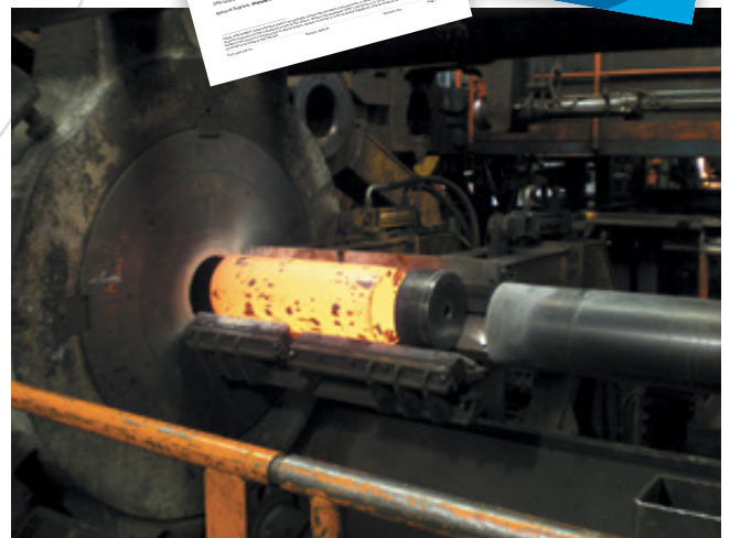
Hot Extrusion of CuNi billet into pipe
