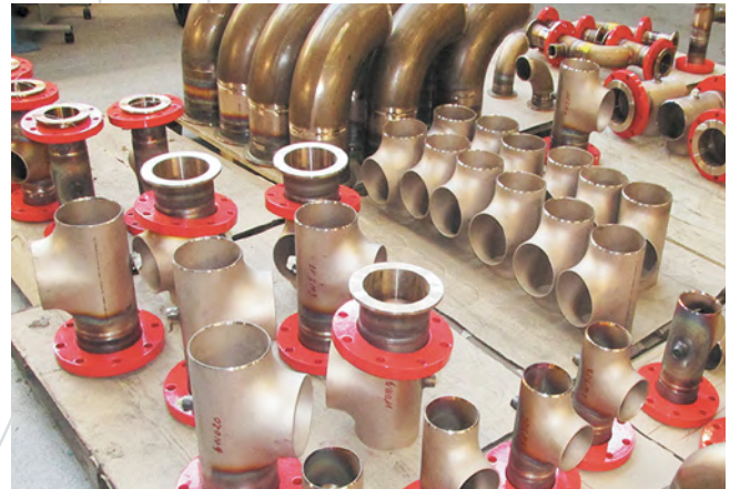
90/10 CuNi piping spools
