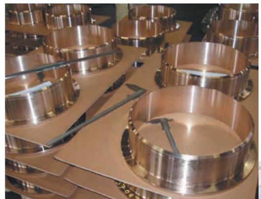
CuNi Inner flanges final inspection
