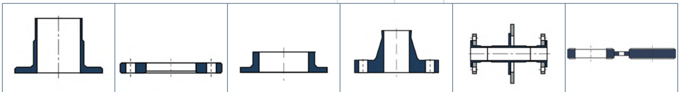
COLLARS/INNER FLANGE LONG TYPE / SHORT TYPE DIN 86037 / EEMUA 234 ASME B 16.9
