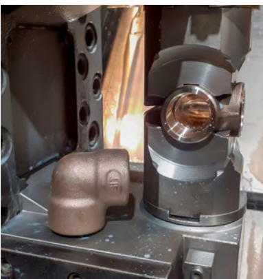
90° socket weld elbow machining
