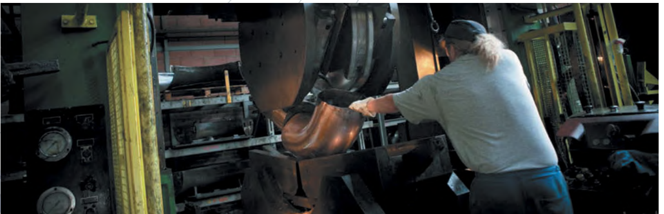
Cold forming CuNi elbows from seamless pipes
