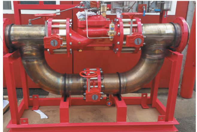
Fire fighting deluge skid 90/10 CuNi
