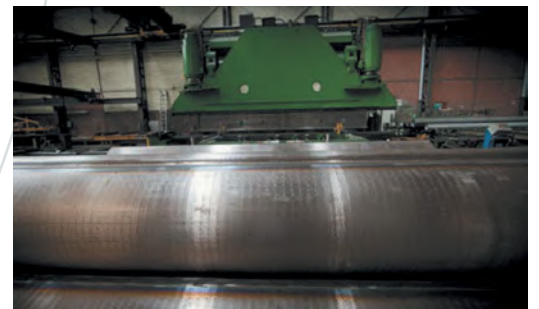
U-BEND PRESS CuNi pipe forming
