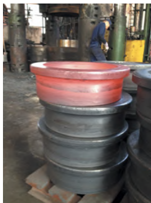
Hot forging of 20" CuNi stub ends
