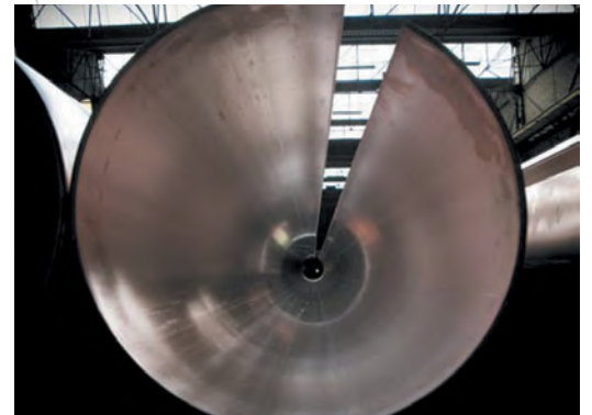
3 ROLLS CuNi pipe forming
