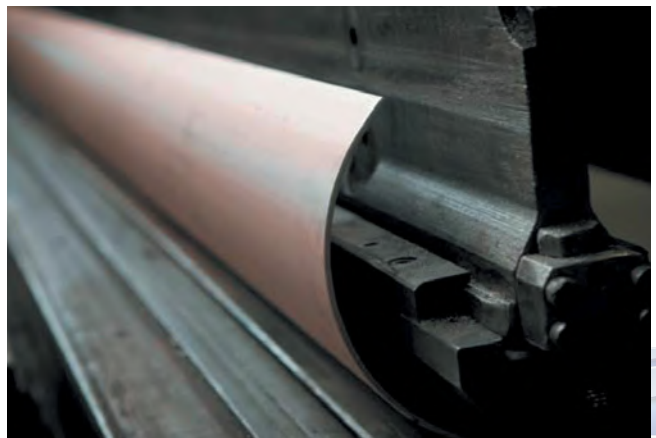
U-BEND PRESS forming CuNi plate into pipe
